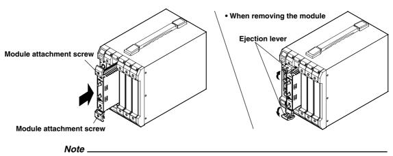
When synchronizing multiple isolated digitizer modules for measurement (module linking), install them in adjacent slots.
